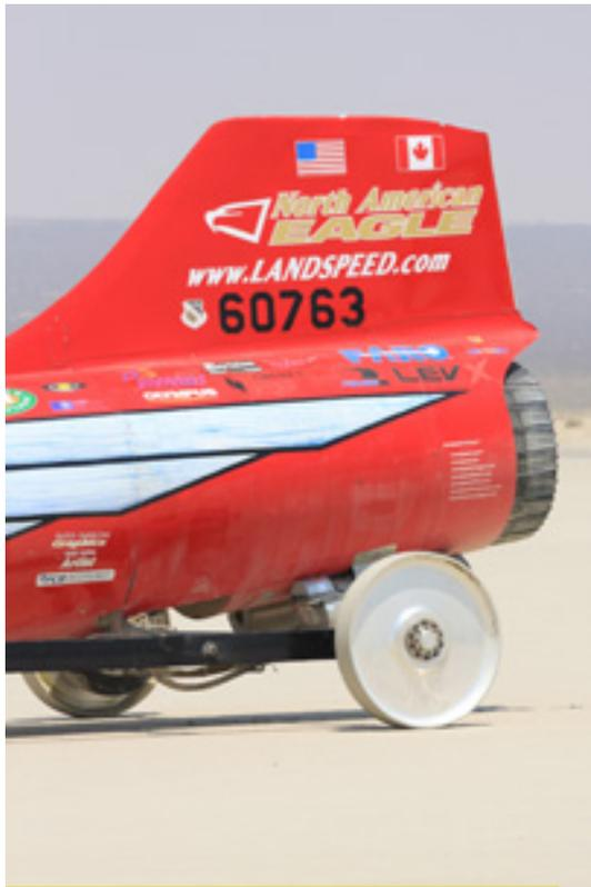
**A non-contacting magnetic brake developed by LevX Technology, part of the rear-wheel assembly, will help slow the NAE vehicle after its 800 mph land speed run.**
