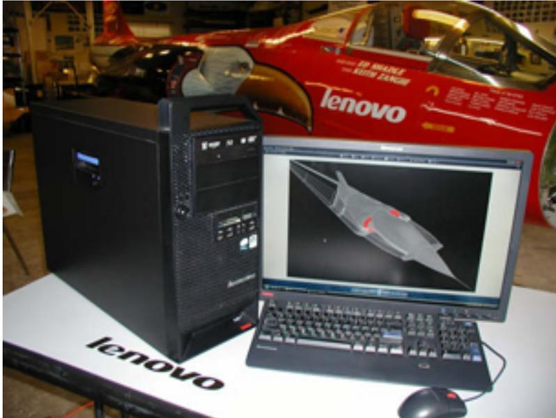
**NAE engineers use the Lenovo ThinkStation D10, running CATIA software, to load the Eagle model and make design changes, as well as collect and analyze performance data after each test run..**
